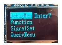
12. Scroll down to the Signal Set and push the SET button to enter the Signal Set menu
