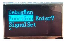
After pushing SET button to enter, there will be a prompt for the password. The factory default password is "006". Push the SET button to enter the password. The password may be changed to another 3-digit number in the configuration menu if required. In this photo, the password has been changed to "000".
