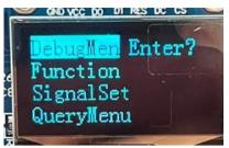
2. Using the DO button to scroll down to "Function" and push the SET button to enter
