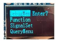
6. Scroll down to the Signal Set and push the SET button to enter the Signal Set menu
