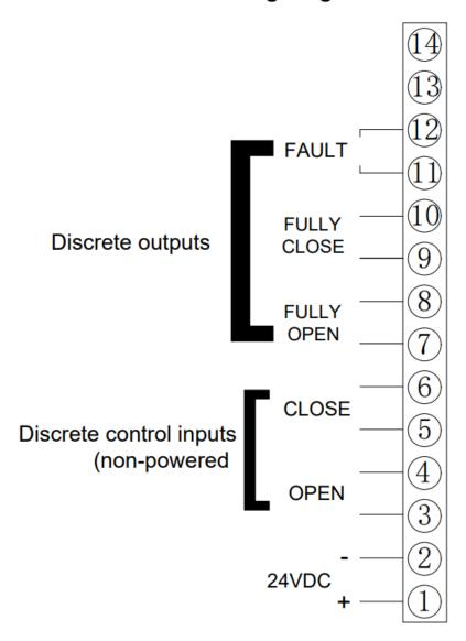
Apply 24 VDC power (+) on 1 and (-) on 2. Insert Control inputs for open/close (on/off) are dry contacts/discrete inputs that ARE NOT POWERED.
